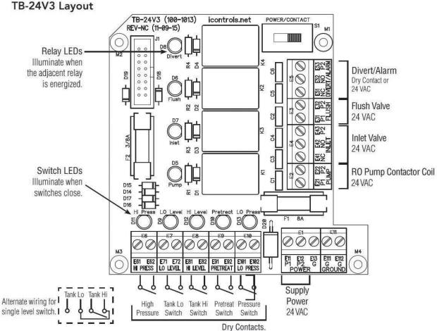
Figure 4-5: Controller Detail: Terminal Board, TB-3
