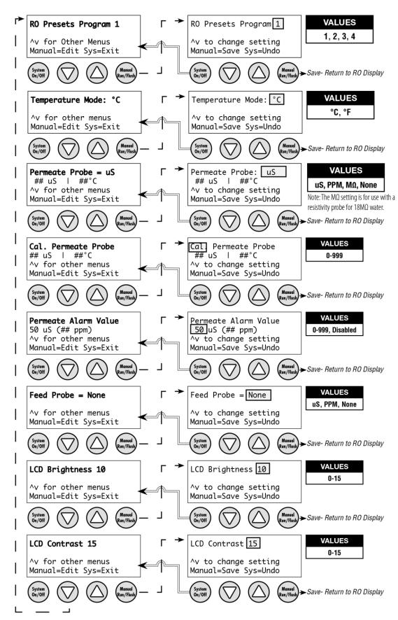
Figure 4-9: Controller Programming: Menu Navigation
