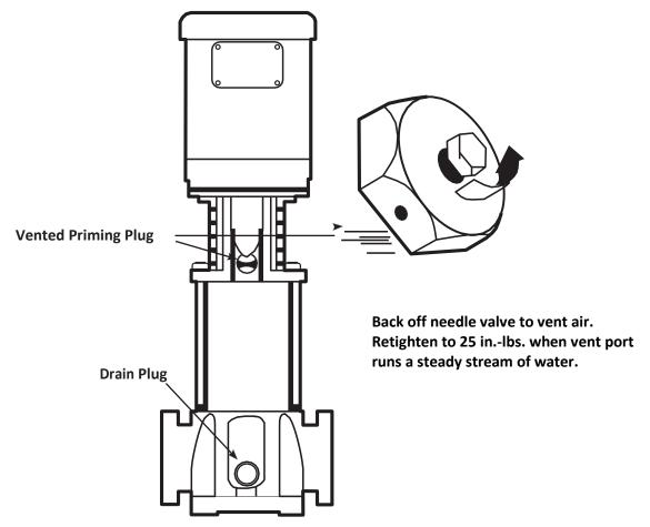
Figure 3-1: Needle Valve Location
