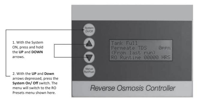
Figure 4-8: Controller Programming. Accessing the hidden menus
