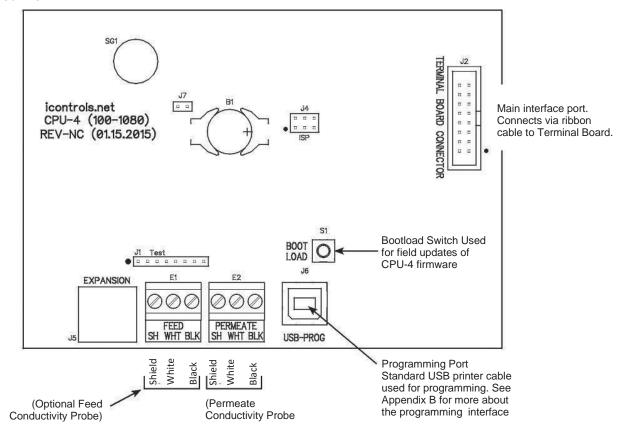
Figure 4-4: Controller Detail: CPU-4
