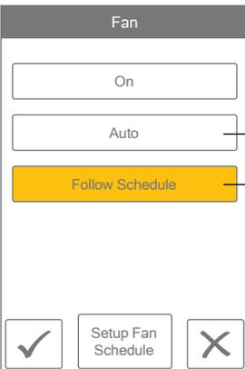
The fan is normally off when set to auto but turns on when needed for the heating or cooling equipment.
