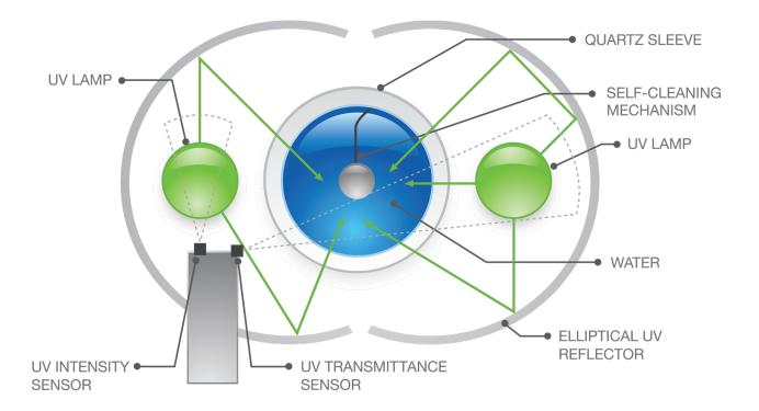
**360° Coverage.** UV-H delivers a sterilizing dose of UV radiation from 360 degrees to overcome shadowing and reliably disinfect water with UVT as low as 35%. Conventional systems require a minimum 75% UVT. In potable water applications this may eliminate the need for water softeners, saving time, money and eliminating salt from drinking water.
